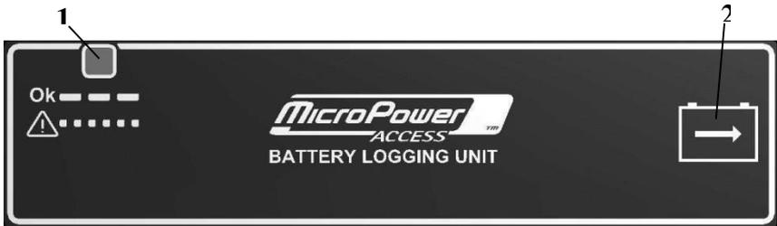
When the BLU is powered up the blue LED will be continuously lit for 2 seconds.
